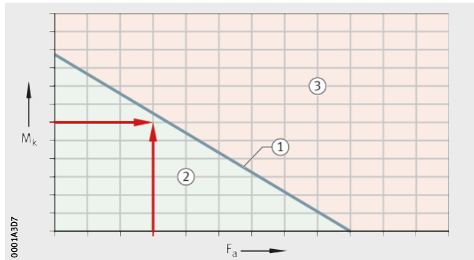
Figure 2 Static limiting load diagram (example)
